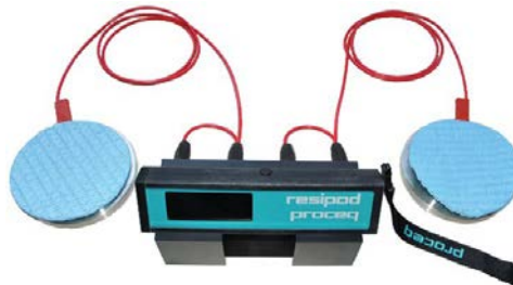
Figure 2: Resipod Proceq concrete resistivity meter
