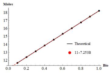
Fig. 3. CO<sub>2</sub> levels as a linear function of the percentage of biofuel
