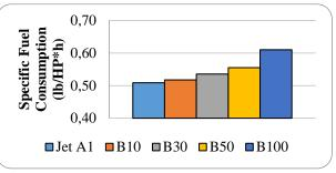
Fig. 6. Comparison of Specific Fuel Consumption
