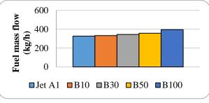
Fig. 7. Comparison of fuel mass flow
