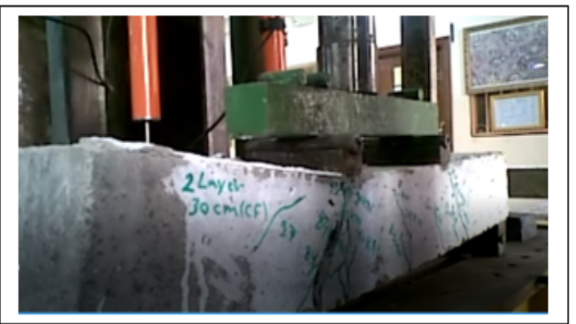
Experimental cracking at failure
