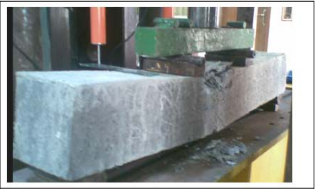
Experimental cracking at failure
