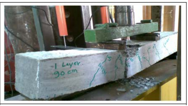
Experimental cracking at failure
