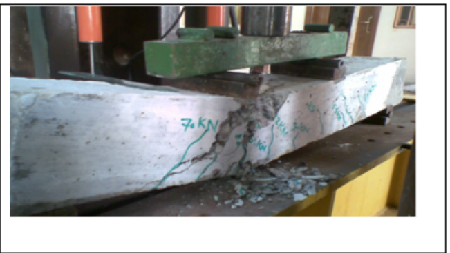
Experimental cracking at failure
