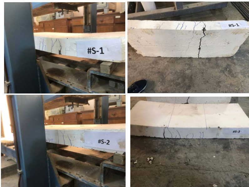
Fig. 10. Failure modes of the tested slabs
