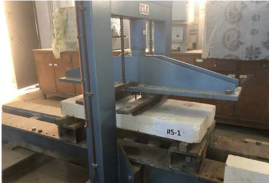
Fig. 8. Slab specimen testing
