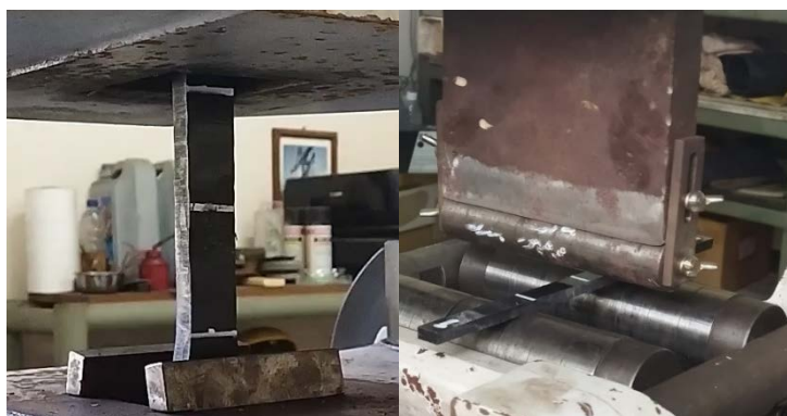
Fig. 3. Tensile and bending test of HDPE Material in material testing laboratory
