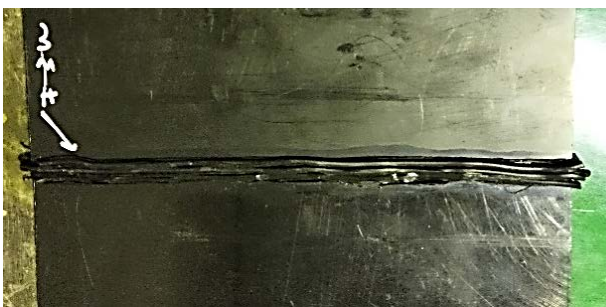
Fig. 6. Welding Results of X Seam Hot Gas Plastic Welding
