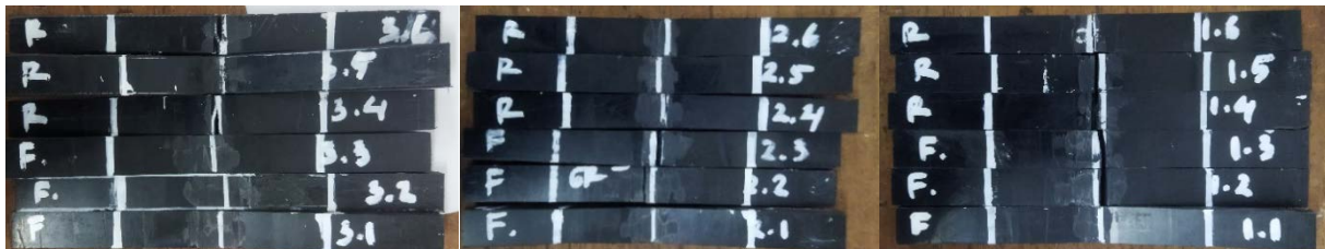
Fig. 13. Fractures of Bending Test Specimens
