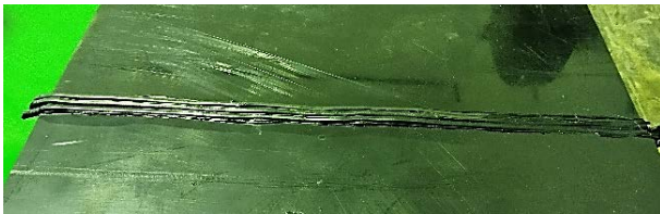
Fig. 5. Welding Results of V-Seam Hot Gas Plastic Welding
