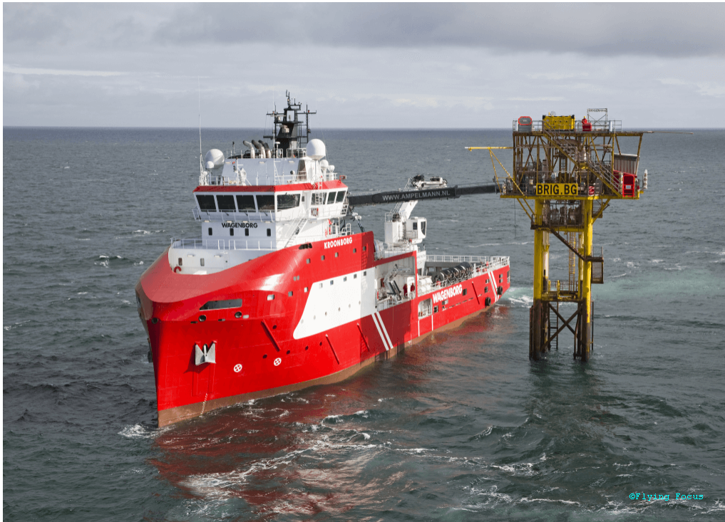
Fig. 5. Supply vessel with walk-to-work system
