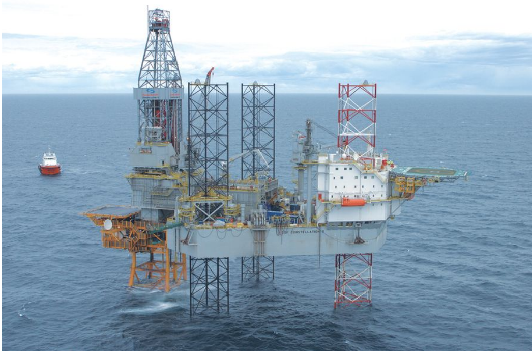
Fig. 2. Example of drilling from the jack-up rig cantilever
