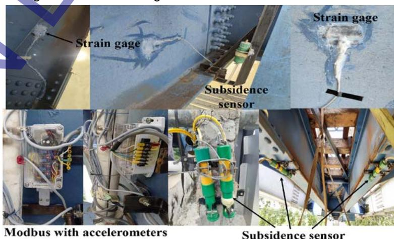
Fig. 3. Placement of subsidence sensors, mod bus with accelerometers, pressure transducer and strain gages
