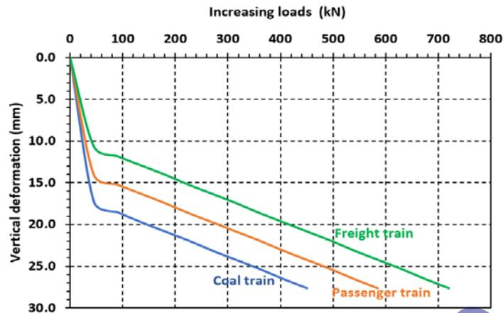
Fig. 9. Numerical simulation results of the maximum deformation of the steel railway bridge under dynamic loads
