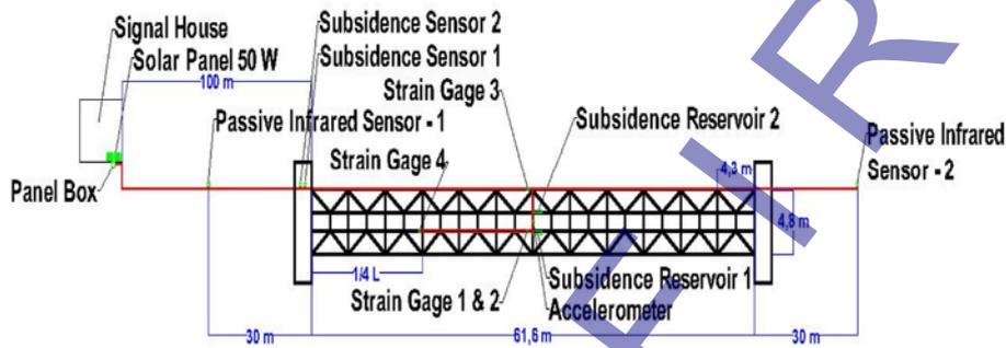
(b) Schematic bottom view of instrumentation location
