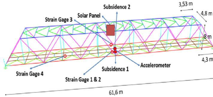
(a) Schematic perspective view of instrumentation locations on the railway bridge
