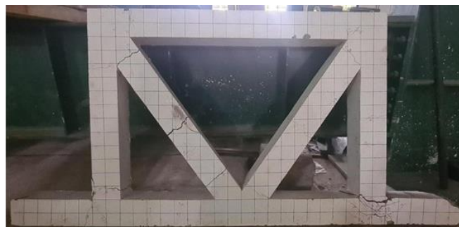
Fig. 15. Failure of CBF structure
