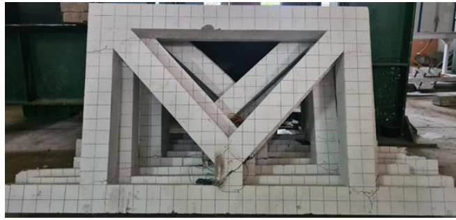
Fig. 16. Failure of EBF shear link of 15 cm structure
