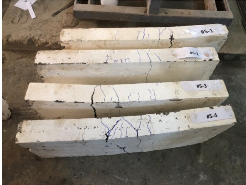
Fig. 9. Failure of solid and hollow slabs (S1, S2, S3, and S4)
