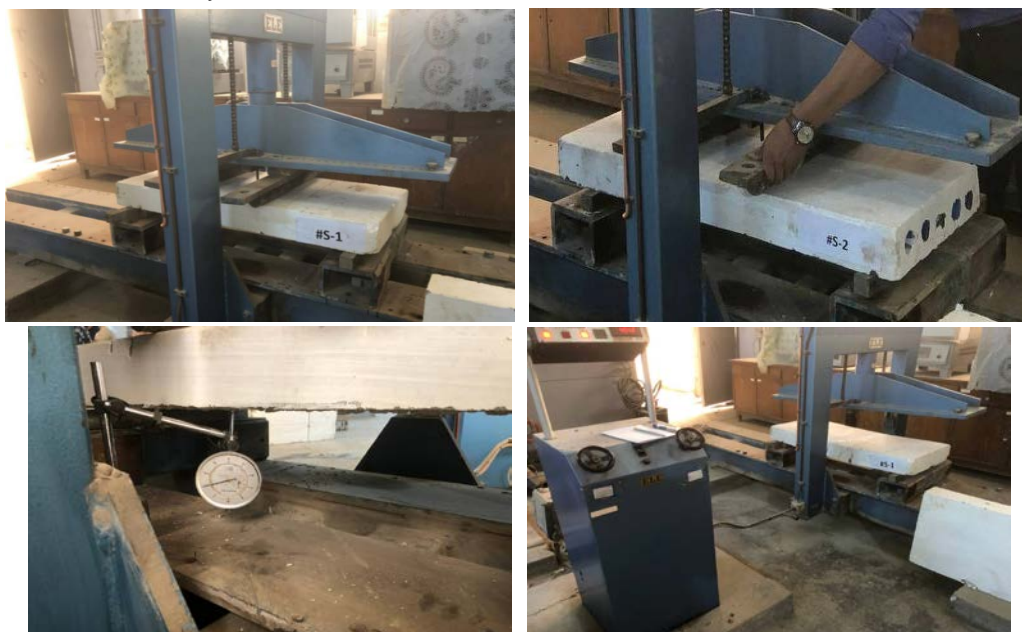
Fig. 8. Preparation of testing slab, diel gage, and universal hydraulic machine
