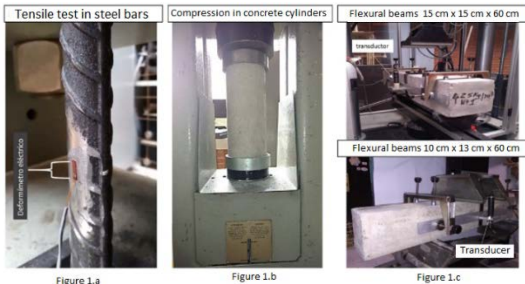
Fig. 2. Laboratory test configuration
