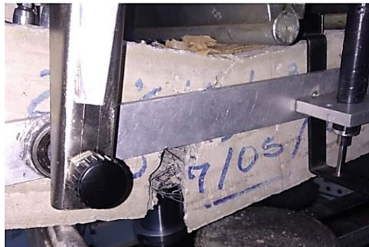
Fig. 12. Type of failure observed in the SFRC beams
