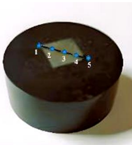
Fig .17. The direction and points of the micro-hardness test
