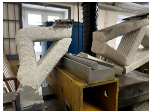
Fig. 9. Failure pattern of a 3D printed girder
