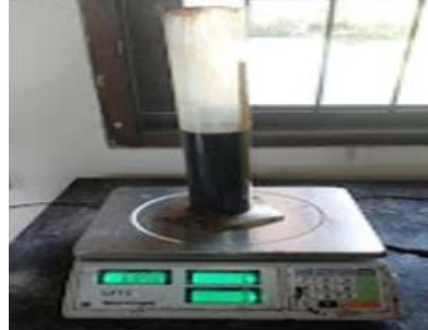
b. Weighing waste engine oil
