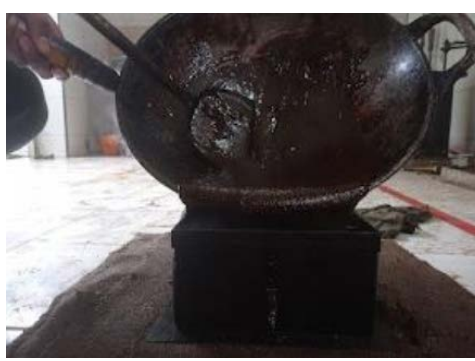
h. Pouring the mixture into a mould
