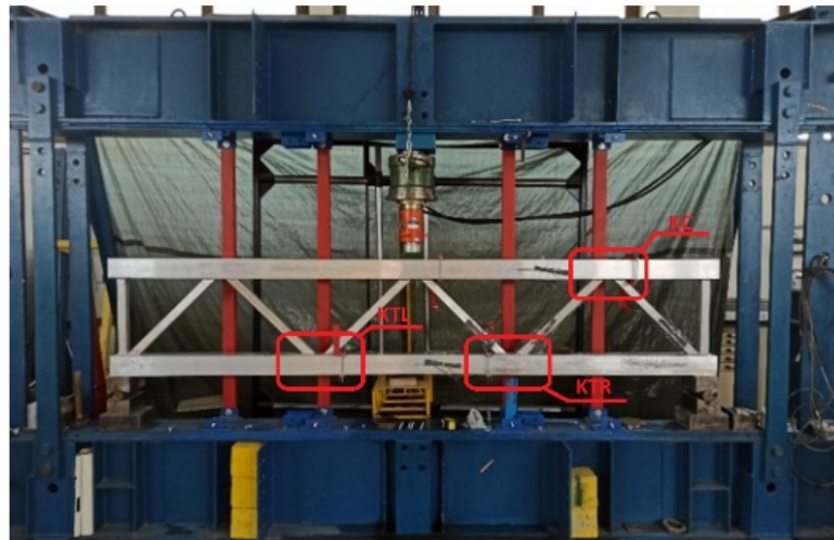
Fig. 5. Welded aluminum joints positioned inside lattice girder
