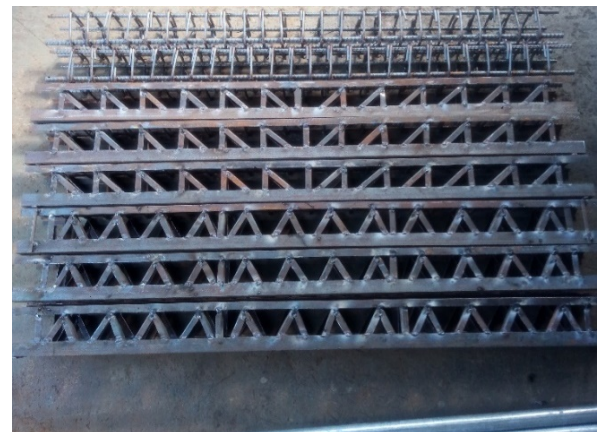
(b) Rebar, Pratt-truss, and Warren-truss models
