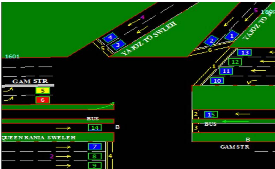
Fig. 6 External patrols intersection adopted from (Sydney Coordinated Adaptive Traffic System (SCATS) from Greater Amman Municipality (GAM))
