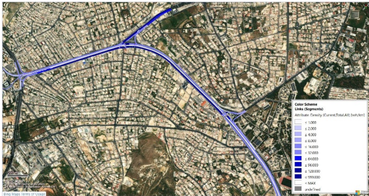
Fig. 14. Density in (vehicle/km) of the whole network for the current situation adopted from PTV Vissim
