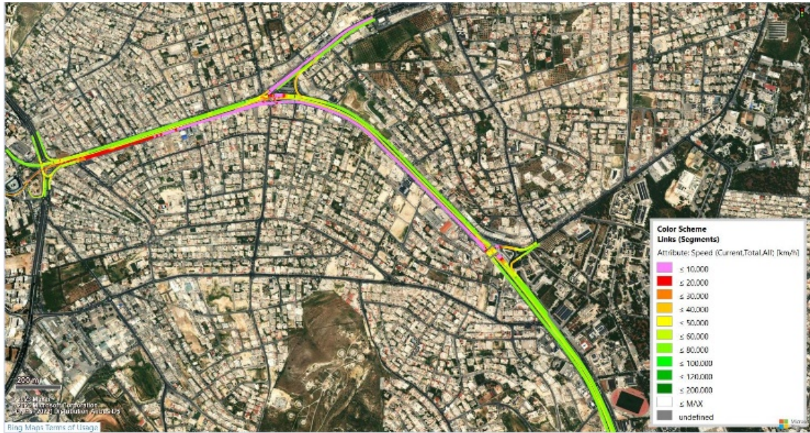
Fig. 13. Vehicles speed in (km/h) for the whole network for the current situation adopted from PTV Vissim
