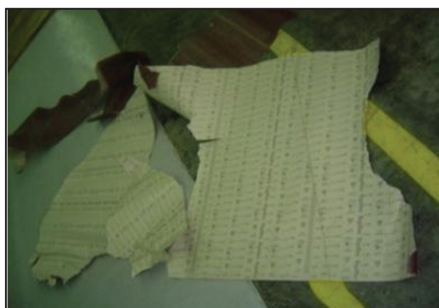
Figure 8: Examples of broken sanding papers
