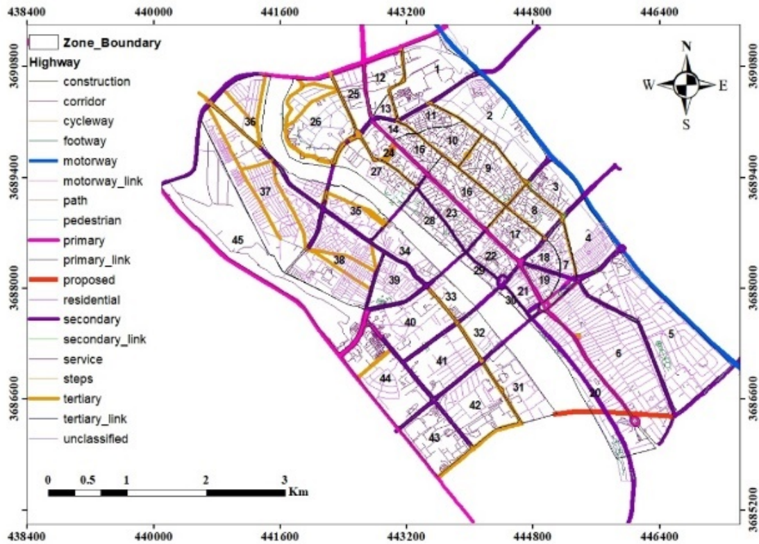
Fig. 3. Illustrates the delineation of zones based on primary, secondary, and tertiary roads, showing the road hierarchy and the classification of road types within each zone
