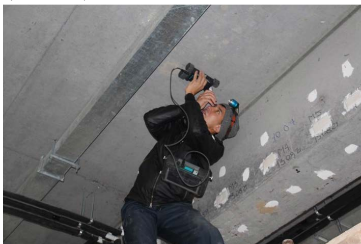
Fig.1 Conducting non-destructive testing of slabs
