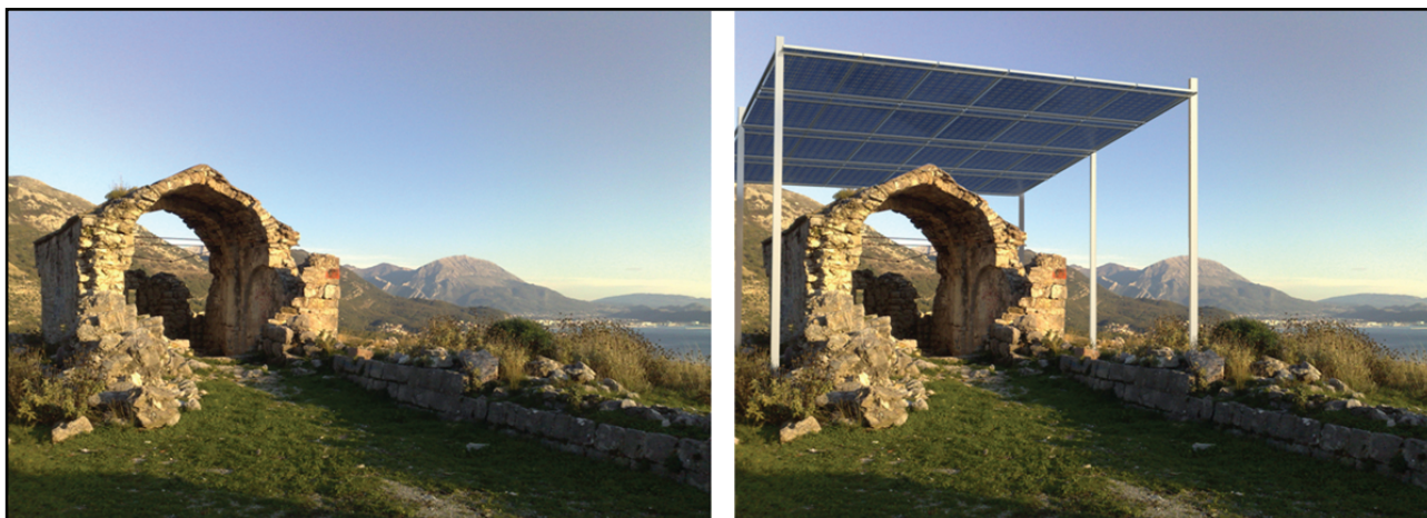
Figure 5: St.Demetrius' Church. Model of building-independent temporary photovoltaic construction (BITPVC)
