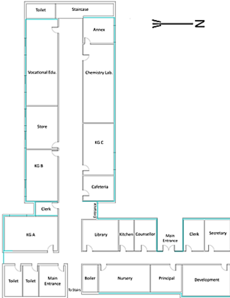
Fig. 4. Ground floor plan of the school (N.T.S.). Blue (thick) lines indicate walls to host 5cm XPS insulation, CMU, and finish layers
