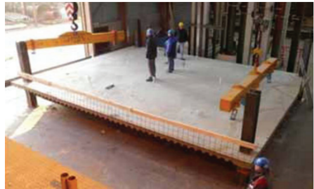
Figure 1: Test setup of FRACOF fire test [11] a) steel elements grid, b) composite floor
