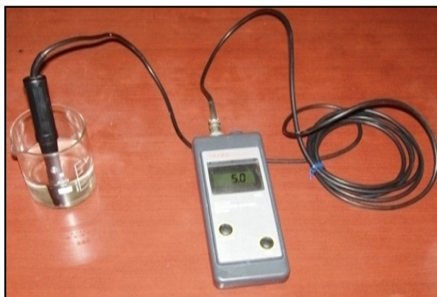
Figure 3: The measuring of oxygen content (HANNA, HI9142 instrument with polarographic sensor after previous calibration [18])
