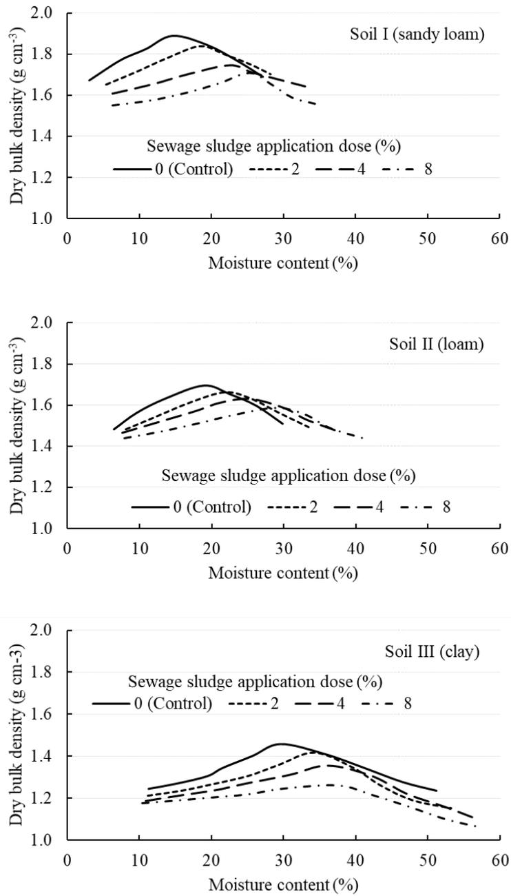
Figure 2. Proctor compaction test curves of soils studied.
