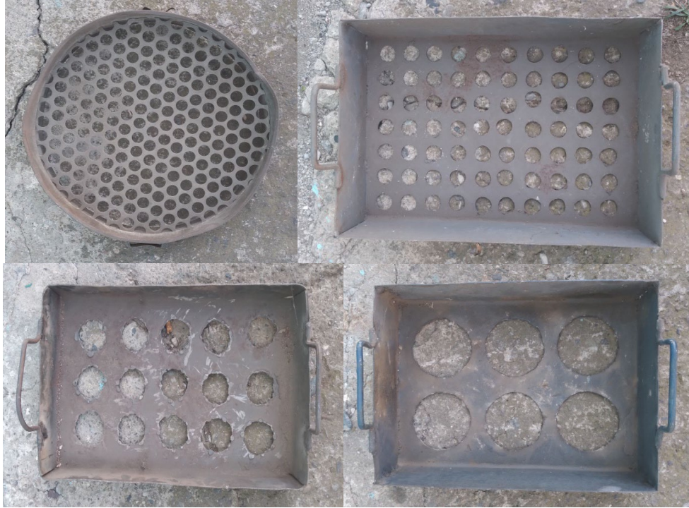
Figure 2. A set of sieves for determining the fractional composition of the soil.
