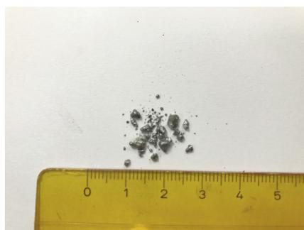
**Figure 11.** Metal particles recovered after the pre-reduction treatment (Mixing D,  $T=1388^{\circ}\text{C}$ ).
