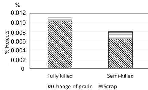
Figure 3. Incidence of rejections classified according to the type of deoxidation used and to the disposition of the rejected material.
