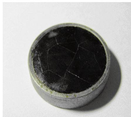
**Figure 1.** Sample 1 in molybdenum crucible after remelting
