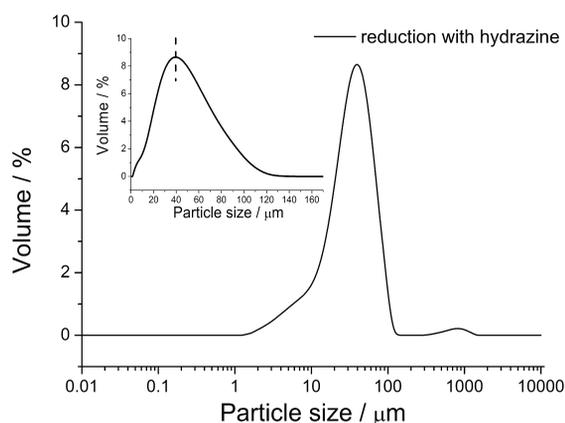
Figure 4. Particle size distribution (PSD) curve for chemically synthesized particles with hydrazine
