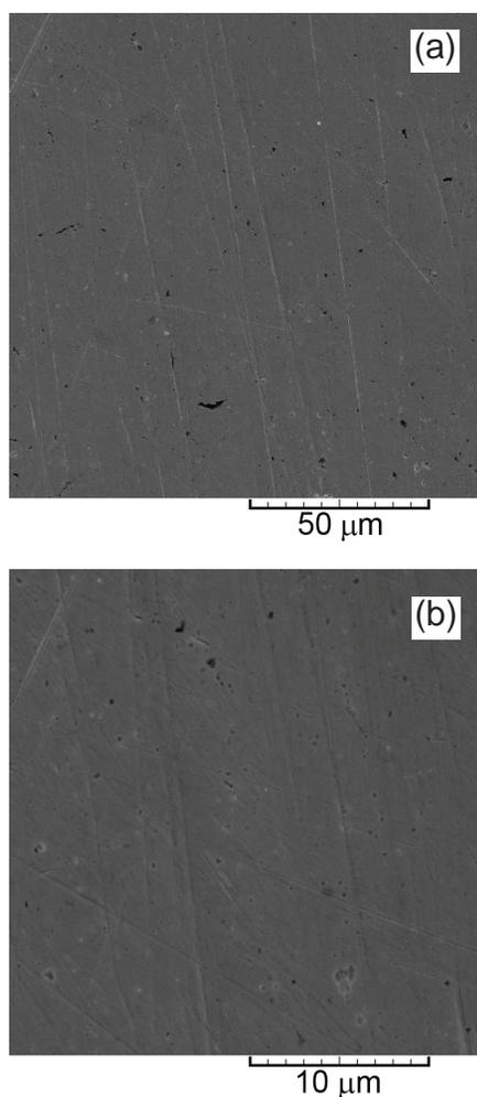
**Figure 1.** The surface area of Pt electrode used in the regimes of galvanostatic and potentiostatic electrolysis of Ag powders. Magnification: (a)  $\times 1000$  and (b)  $\times 5000$
