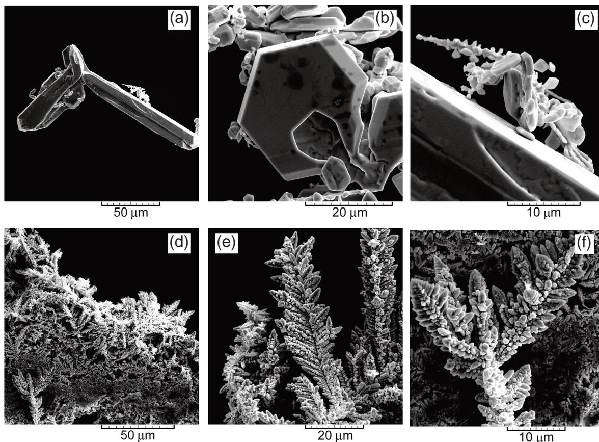
**Figure 7.** Morphologies of particles produced galvanostatically using: a) – c) the NIT solution, magnification: (a)  $\times 800$ , (b)  $\times 3000$ , (c)  $\times 5000$ ;  $t = 246$  s, and d) – f) the AM solution, magnification: (d)  $\times 1000$ , (e)  $\times 2000$ , (f)  $\times 4000$ ;  $t = 266$  s
