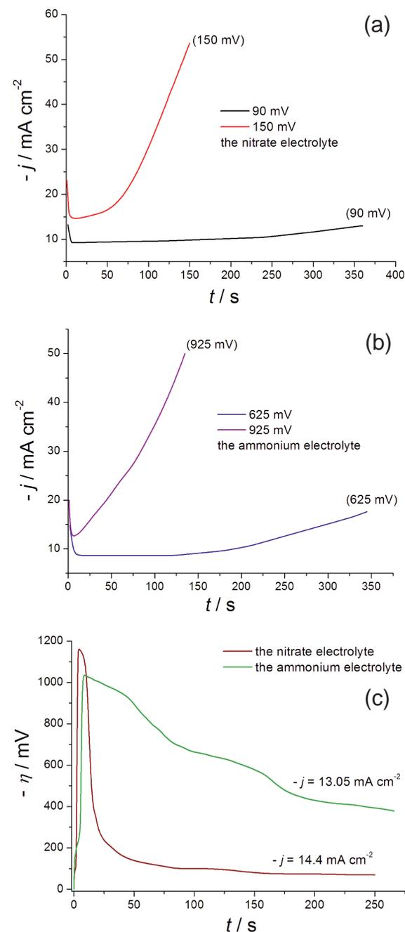
**Figure 3.** The chronoamperometric curves obtained from: a) the NIT solution, b) the AM solution, and c) the chronopotentiometric curves obtained from NIT and AM solutions
