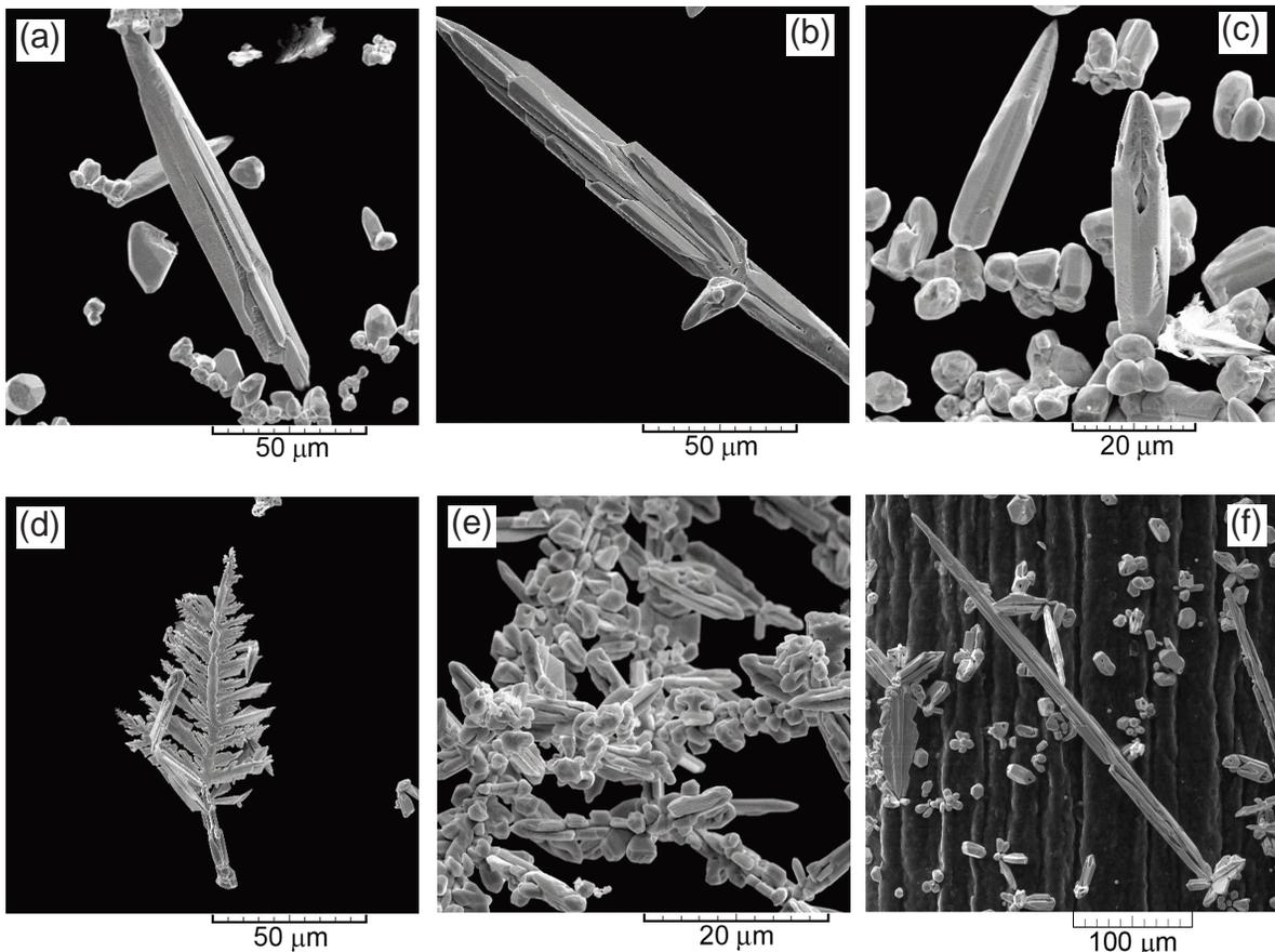
**Figure 9.** Morphologies of powder particles obtained potentiostatically using the NIT solution at overpotentials of: a) – c)  $-90$  mV, magnification: (a)  $\times 1000$ , (b)  $\times 1000$ , (c)  $\times 2000$ ;  $t = 360$  s, d) – f)  $-150$  mV, magnification: (d)  $\times 1000$ , (e)  $\times 3000$ , (f)  $\times 600$ ;  $t = 150$  s
