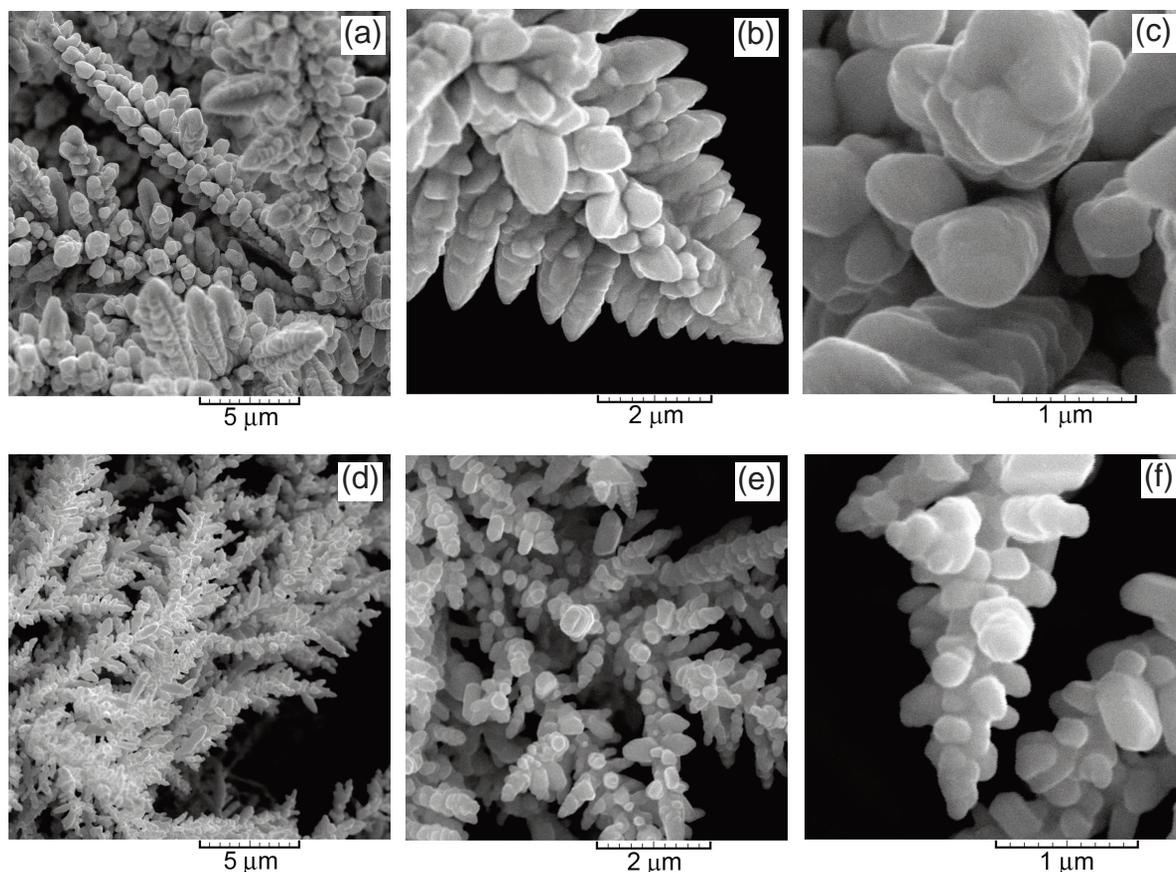
**Figure 11.** Morphologies of particles produced potentiostatically using the AM solution at overpotentials of: a) – c)  $-625$  mV, magnification: (a)  $\times 7000$ , (b)  $\times 20000$ , (c)  $\times 50000$ ;  $t = 345$  s, and d) – f)  $-925$  mV, magnification: (d)  $\times 7000$ , (e)  $\times 20000$ , (f)  $\times 50000$ ;  $t = 135$  s
