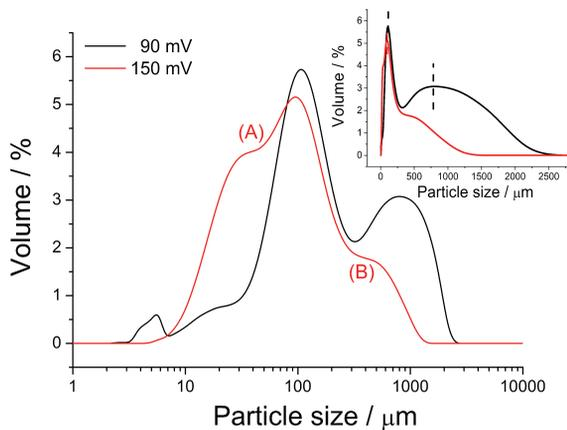
**Figure 8.** Particle size distribution (PSD) curves for Ag particles produced in the POT regime by use of the NIT solution at  $-90$  and  $-150$  mV
