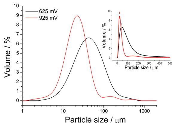
**Figure 10.** Particle size distribution (PSD) curves for Ag particles obtained potentiostatically using the AM solution at  $-625$  and  $-925$  mV
