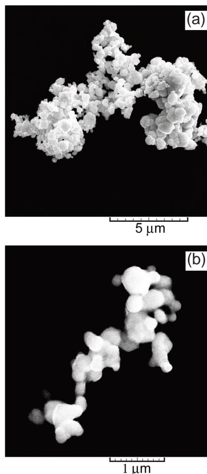
Figure 5. Morphologies of chemically synthesized Ag powder particles obtained by reduction with hydrazine. Magnification: (a)  $\times 10000$  and (b)  $\times 35000$
