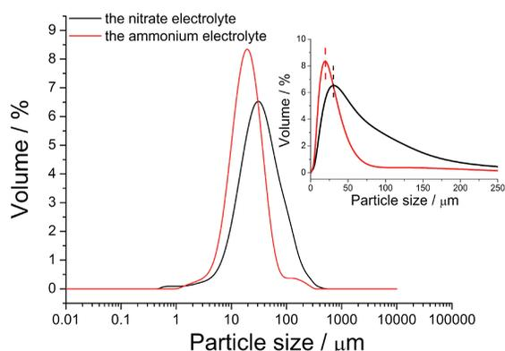
**Figure 6.** Particle size distribution (PSD) curves for Ag particles obtained galvanostatically by use of the NIT and the AM solutions
