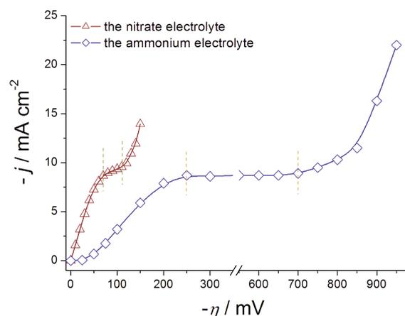
**Figure 2.** The polarization curves for Ag electrodeposition from the NIT and the AM solutions. According to Ref. [10]
