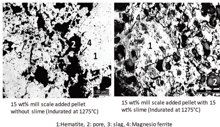
**Figure 12.** Optical microstructure of mill scale added basic pellet (0.3 basicity) with and without the addition of iron ore slime
