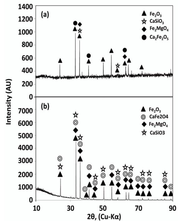
**Figure 11.** XRD of mill scale added basic pellet (0.3 basicity) with and without the addition of iron ore slime (a) 15 wt% mill scale added pellet without slime (indurated at 1275°C) (b) 15 wt% mill scale added pellet with 15% slime (indurated at 1275°C)
