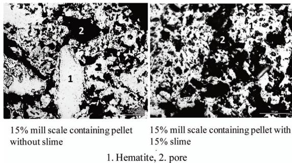
**Figure 6.** Optical microstructure of mill scale added acidic pellets with and without addition of iron ore slime
