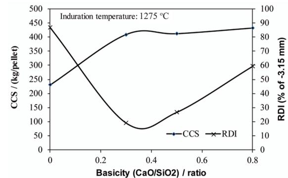
**Figure 4.** Effect of Basicity on CCS and RDI of indurated fluxed pellet
