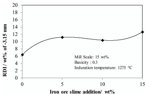
Figure 13. Effect of iron ore slime addition on RDI of mill scale added basic hematite pellet
