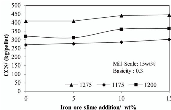
**Figure 9.** Effect of iron ore slime addition on the CCS of mill scale added basic hematite pellet
