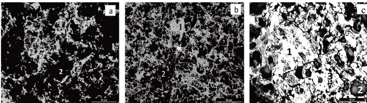
Figure 14. Optical microstructure of mill scale added basic pellet (0.3 basicity) with addition of iron ore slime (15wt%) at different temperature; 1 - Hematite, 2- Pore, 3 - Slag; (a) 1175 °C induration, (b) 1200 °C induration, (c) 1275 °C induration
