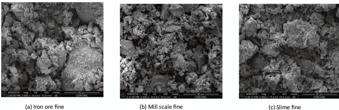
Figure 2. Surface morphology of different fines under SEM microscope
