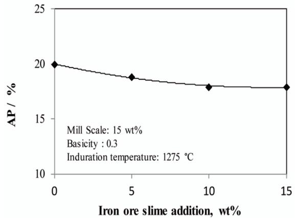
**Figure 10.** Effect of iron ore slime addition on the AP of mill scale added basic hematite pellet
