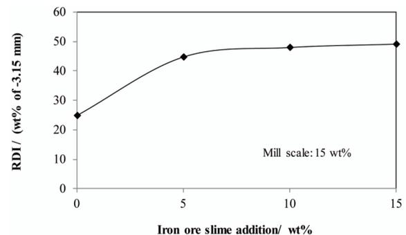
**Figure 8.** Effect of iron ore slime addition on RDI of mill scale added hematite pellet
