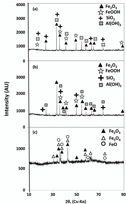
**Figure 1.** XRD analysis of iron ore, slime and mill scale; (a) iron ore, (b) iron ore slime, (c) mill scale
