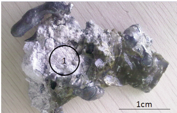
Figure 1. A node attached to the SEN causing the clogging (the sample taken in the black circle)
