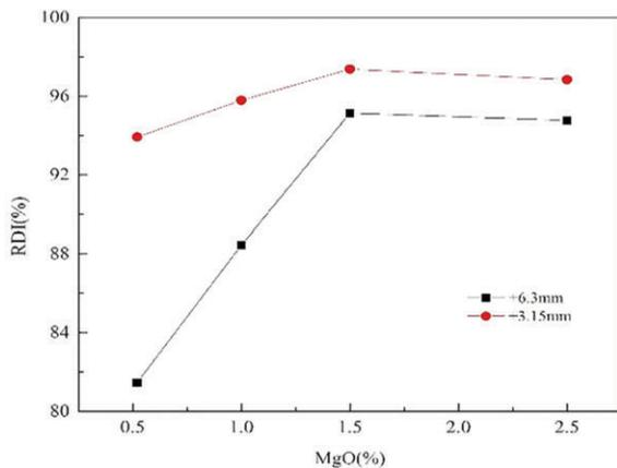
Figure 7. Influence of MgO content on RDI of fired pellets in the mini scale
