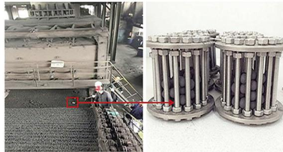
Figure 8. Cages containing the green pellets were loaded into the chain grate
