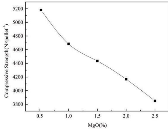
Figure 1. Influence of MgO content on the compressive strength of pellets in the mini scale (Preheating at 1198K (925°C) for 12min and roasting at 1473K (1200°C) for 9min)
