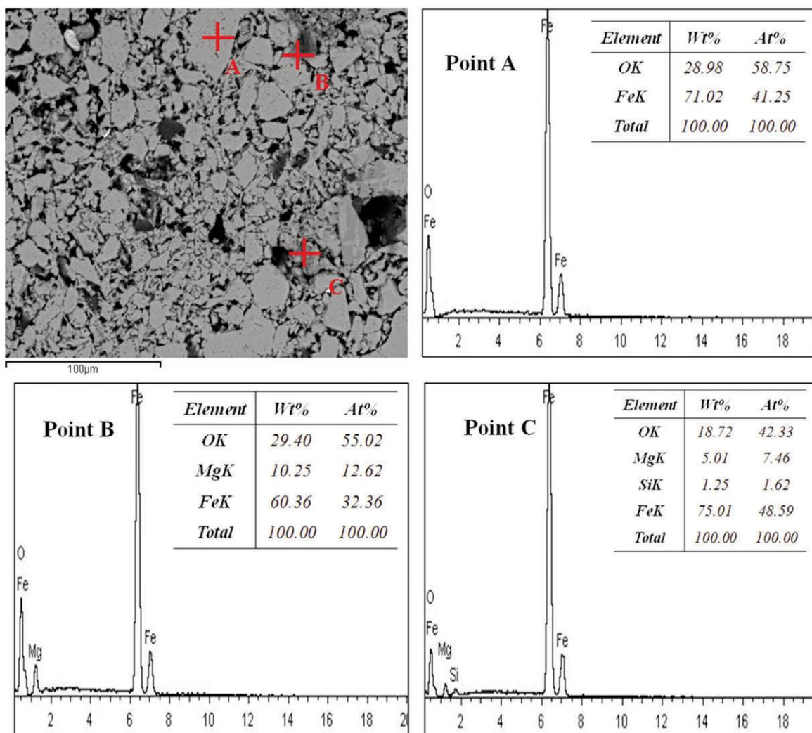
Figure 4. The SEM-EDS of fired pellets with 2.50% MgO
