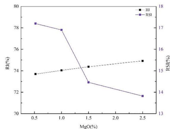
Figure 5. Influence of MgO content on RI and RSI of fired pellets in the mini scale
