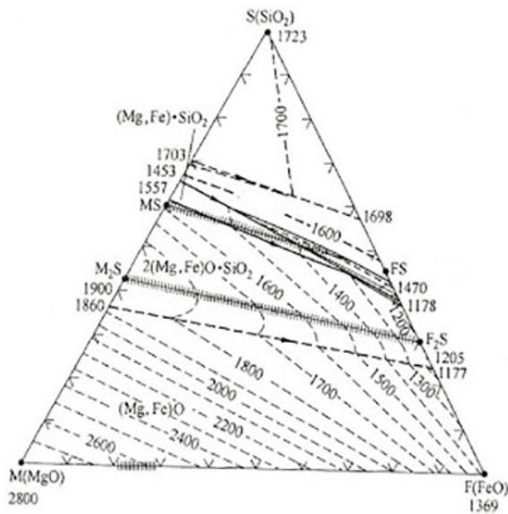
Figure 6. FeO-MgO-SiO<sub>2</sub> ternary phase diagram
