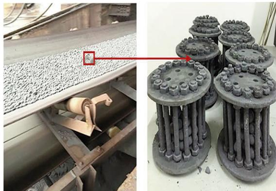
Figure 9. Cages containing the fired pellets were recovered from the belt after cooling machine
