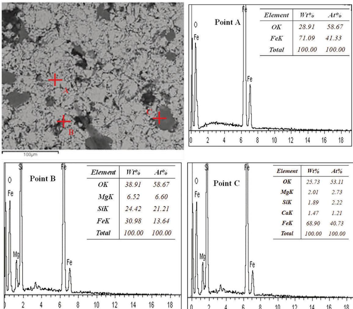
Figure 3. The SEM-EDS of fired pellets with 1.50%  $\text{MgO}$
