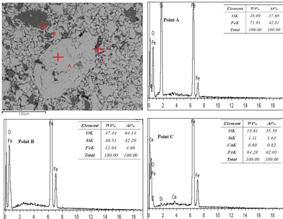
Figure 2. The SEM-EDS of fired pellets with 0.52% MgO without adding magnesite
