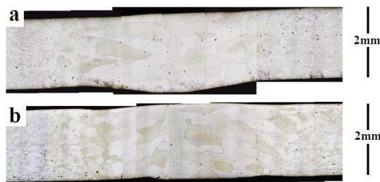
Figure 4. The effect of welding current on the weld pool shape of the similar joints, a) sample S6, b) sample S4.
