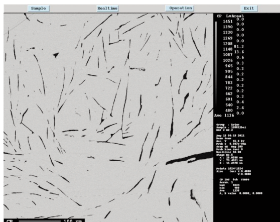
Figure 6. SEM micrograph of the metal phase from the second test. The dark stripes in the metal matrix consist of carbon.
