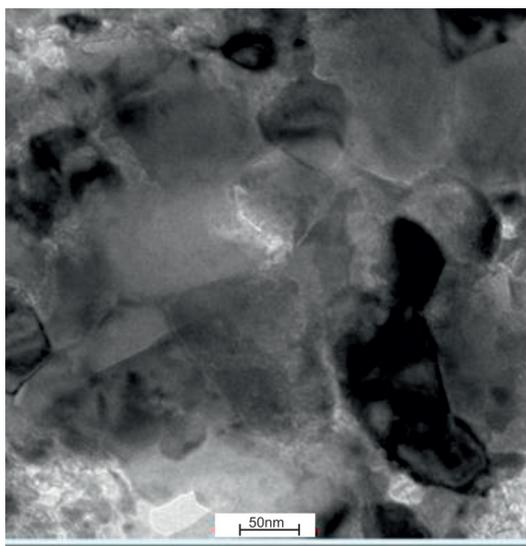
**Figure 9.** Microstructure of ZnAlCu0.1Mg alloy, micrograins Zn, HAADF
