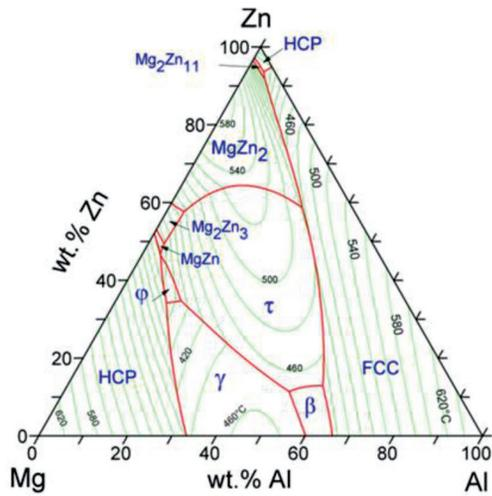
Figure 1. Liquidus projection of the Mg-Al-Zn system [9]
