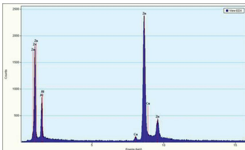
**Figure 11.** EDS microanalysis of the area presented in Fig. 10
