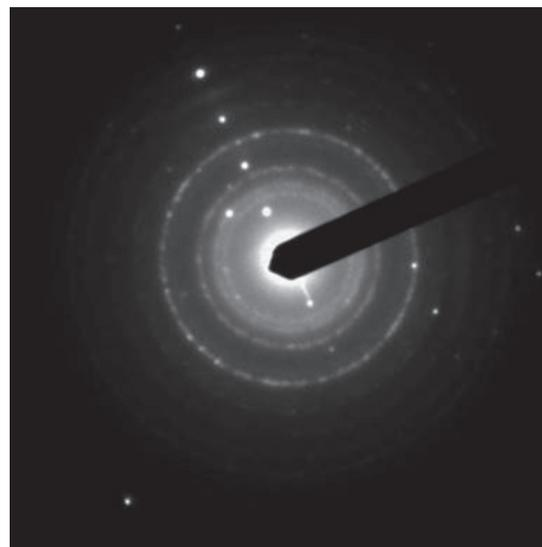
**Figure 8.** Electron diffraction of the area in fig. 7, polycrystalline Zn phase structure
