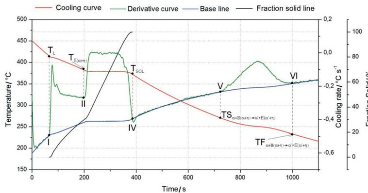
Figure 3. Cooling curve, derivative curve, base line, and fraction solid (FS) of ZnAlCu alloy
