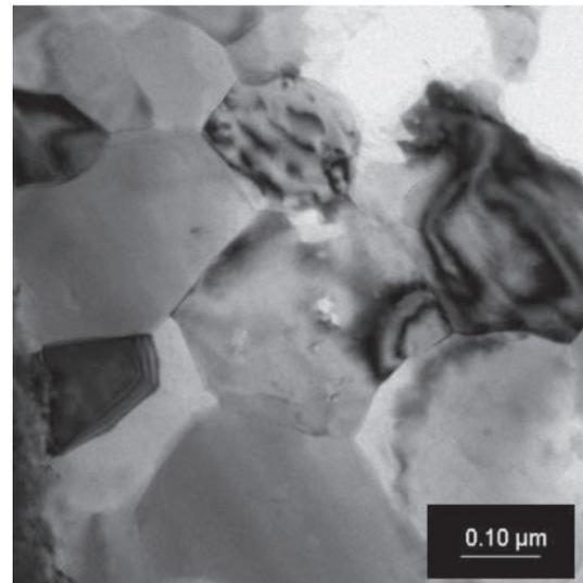
**Figure 7.** Microstructure of ZnAlCu0.1Mg alloy, micrograins Zn, TEM bright field
