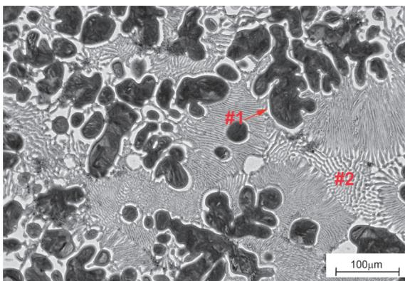
**Figure 5.** Microstructure of Zn-10Al-1Cu alloy: #1 – phase  $\alpha'$ , #2 – eutectic  $\alpha'+\eta$
