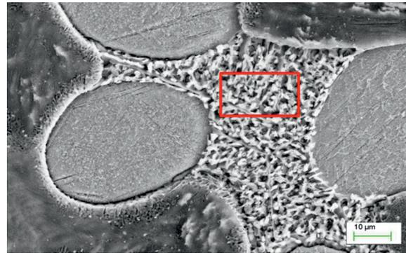
**Figure 6.** Microstructure of Zn-8Al-0.8Cu-0.1Mg, mass concentration of elements in the marked area: Mg – 1.84 % wt.; Al – 23.9 % wt.; Zn – ballance
