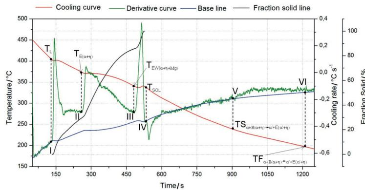
Figure 2. Cooling curve, derivative curve, base line, and fraction solid (FS) of ZnAlCu alloy with addition of 0.1% wt. Mg
