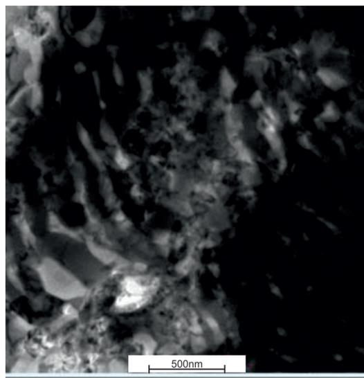
**Figure 10.** Microstructure of ZnAlCu0.1Mg alloy, Zn eutectics, HAADF
