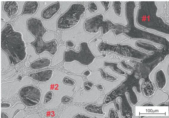
**Figure 4.** Microstructure of Zn-8Al-0.8Cu alloy with addition of 0.1% wt. Mg: #1 – phase  $\alpha'$ , #2 – phase  $\eta$ , #3 – eutectic with Mg
