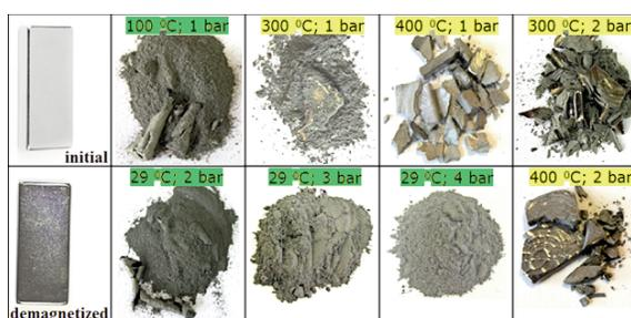
**Figure 3.** Initial, demagnetized and disintegrated magnets; dark grey captions indicates those samples which are indicated as fully disintegrated
