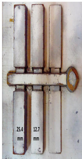
Figure 4. Pattern which contains 6 plates of 120 x 40 mm and a thickness ranging from 25.4 to 4.23 mm
