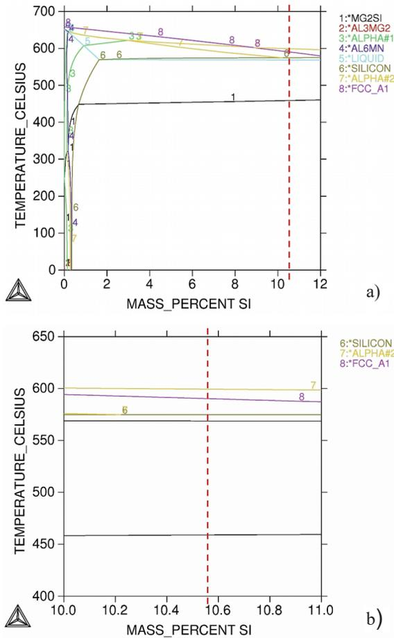
Figure 3. Equilibrium phase diagram of investigated AlSi9MgMn alloy: a) Aluminum corner 0-12 wt.%Si, 0-700 °C, b) Aluminium corner cut 10-11 wt.%Si, 400-650 °C
