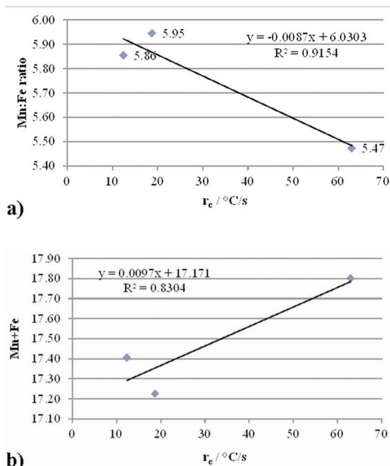
**Figure 7.** Influence of cooling rate on  $Al_{15}(Mn,Fe)_3Si_2$  phases morphology development: a) (Mn:Fe) ratio and b) Mn+Fe values
