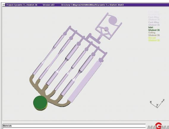
Figure 2. Casting geometry for HPDC used for simulation with MAGMASOFT software
