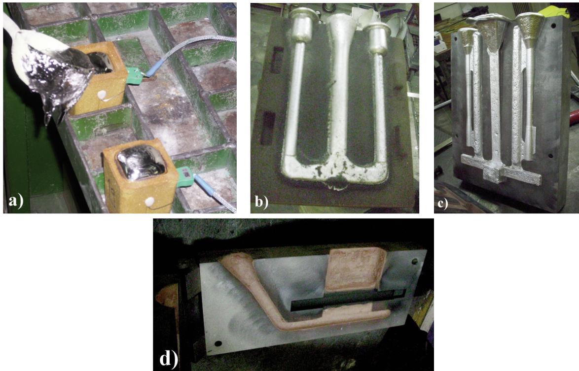
**Figure 1.** Mould types used for achieving different cooling rates: a) Croning cell (3 °C/s), b) Sand mould (12.4 °C/s), c) Permanent mould - ASTM B108 mould (18.7 °C/s), d) Permanent mould (21.5 °C/s)
