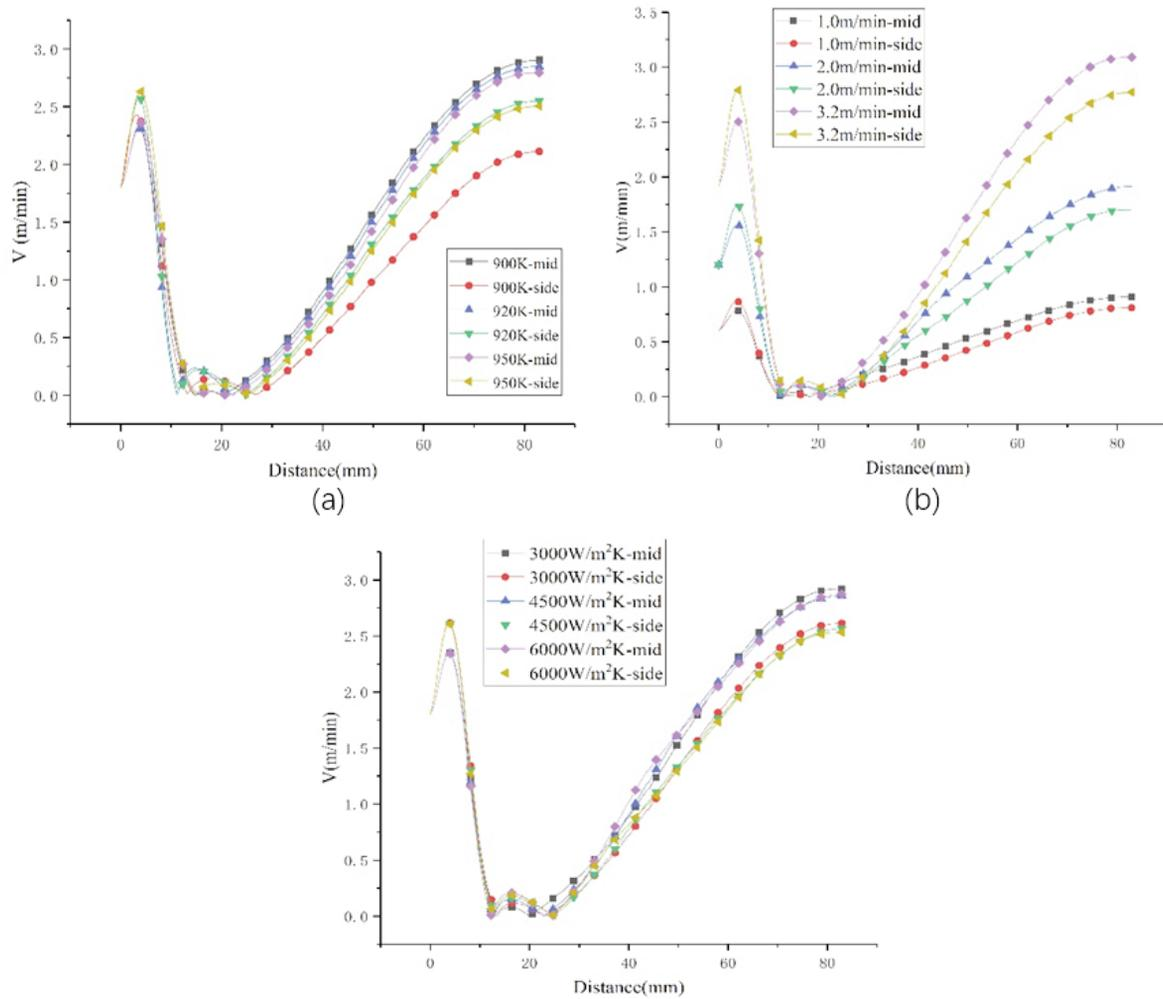
**Figure 6.** Velocity diagram of center line and edge line in cast rolling area: (a) Different casting and rolling temperature velocity diagram; (b) Different casting and rolling speed diagram; (c) Different heat transfer capacity speed diagram
