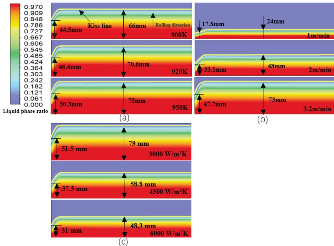
Figure 4. Liquid fraction nephogram of casting and rolling zone with different process parameters: (a) Liquid fraction nephogram of different casting and rolling temperature; (b) Liquid fraction nephogram of different casting and rolling speed; (c) Liquid fraction nephogram of different heat transfer capacity
