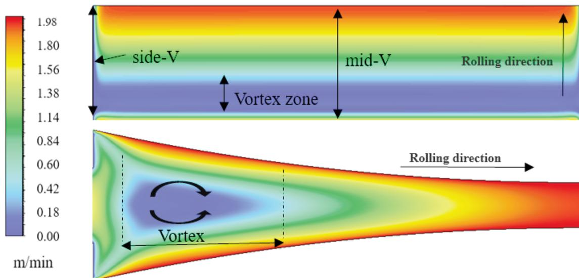
Figure 5. Velocity field and eddy current in casting rolling area
