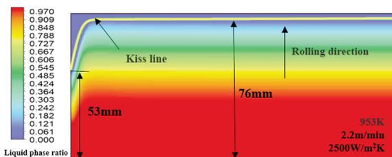
Figure 9. Nephogram of liquid phase ratio of optimum process parameters
