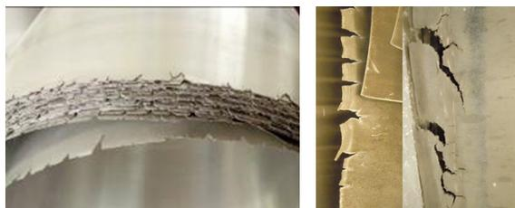
Figure 1. Defects in magnesium alloy cast-rolled strip
