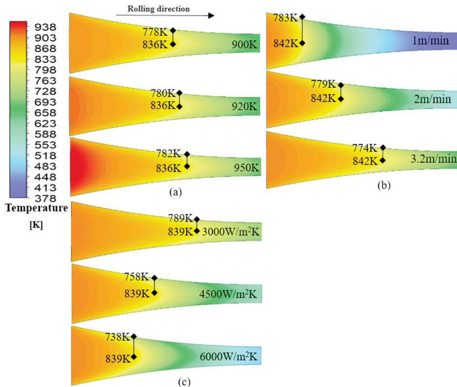
**Figure 7.** Temperature nephogram of casting and rolling area edge: (a) Edge temperature nephogram of different casting and rolling temperature; (b) Edge temperature nephogram of different casting and rolling speed; (c) Edge temperature nephogram of different heat transfer
