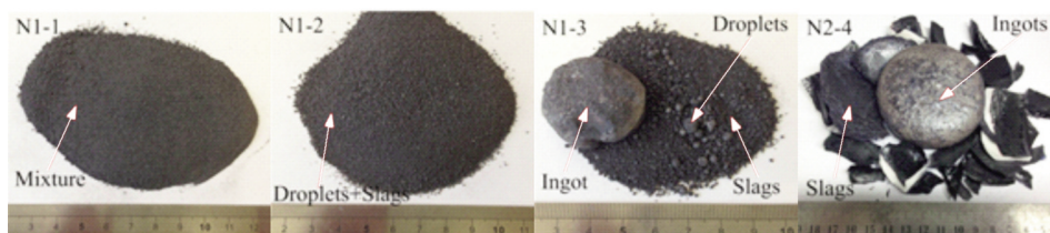
Figure 6. Samples (N1-1, N1-2, N1-3, N2-4) obtained after induction furnace experiments.
