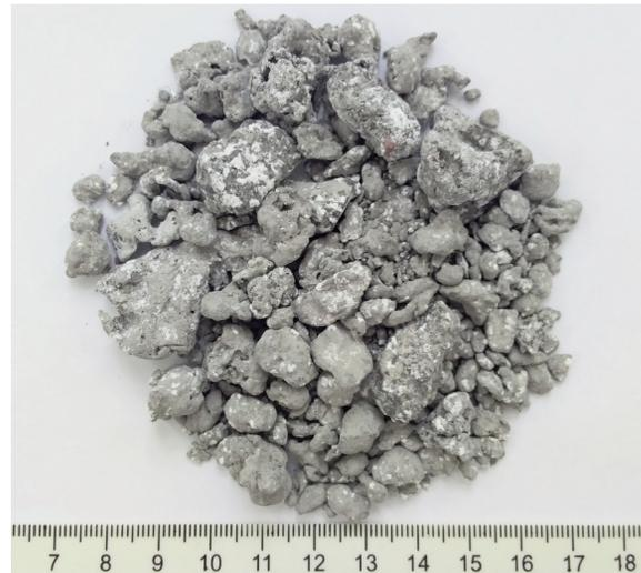
Figure 1. Shape of the used aluminum slags
