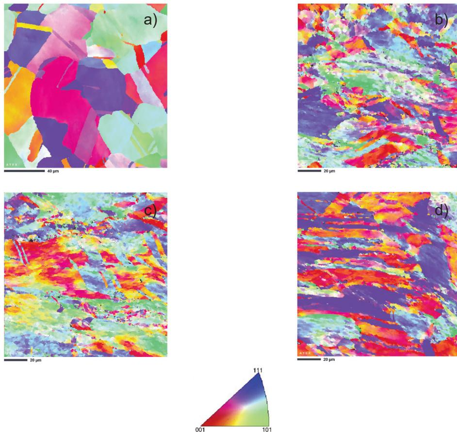
**Figure 7.** IPF-Z maps of the CuCoNi alloy: a) after supersaturation, b) ECAP 100  $^\circ\text{C}$ , c) ECAP 200  $^\circ\text{C}$ , d) ECAP 250  $^\circ\text{C}$
