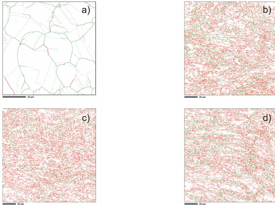
**Figure 8.** Maps of the grain boundary misorientation: a) after supersaturation, b) ECAP 100 °C, c) ECAP 200 °C, d) ECAP 250 °C (red - low-angle boundaries 3-15°, green - high-angle boundaries 15-58°, grey - twin boundaries 58-63.5°)
