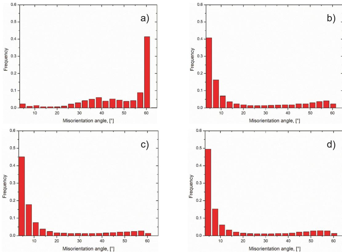
**Figure 9.** Misorientation angle distributions for the CuCoNi samples a) after supersaturation, b) ECAP 100 °C, c) ECAP 200 °C, d) ECAP 250 °C
