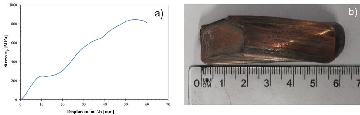
**Figure 3.** a) The forces registered in the ECAP process for sample no. 2 at 100 ° C; b) sample after the completed ECAP process
