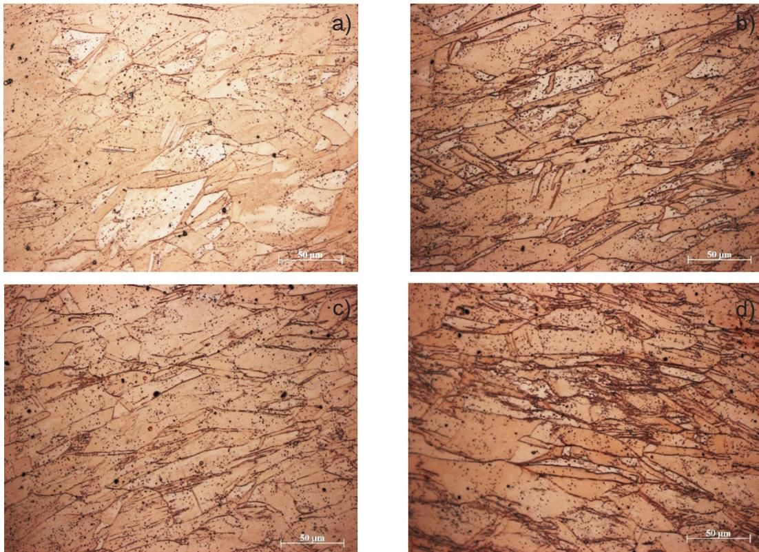
**Figure 6.** Microstructure of the CuCoNi alloy after the ECAP process at the temperature: a) 20/200 °C, b) 100 °C, c) 200 °C, d) 250 °C
