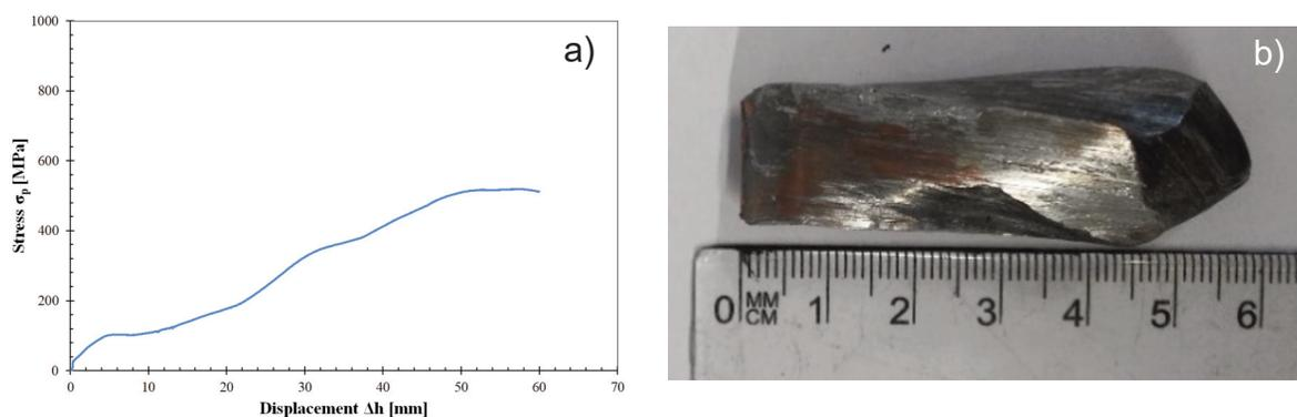
**Figure 4.** a) The forces registered in the ECAP process for sample no. 3 at 200 ° C; b) the sample after the completed ECAP process
