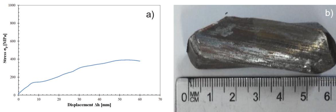
**Figure 5.** a) The forces registered in the ECAP process for sample 4 at 250 ° C; b) sample after the completed ECAP process
