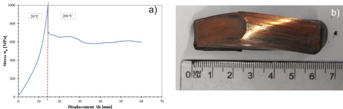
**Figure 2.** a) The forces registered in the ECAP process for sample no. 1 at 20 °C / 200 °C, b) sample after the completed ECAP process
