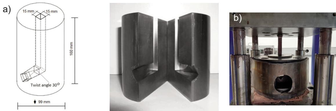
**Figure 1.** ECAP die with a modified output channel: a) construction diagram, image of the die, b) the entire arrangement of the tool
