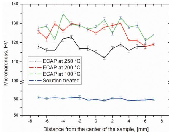
Figure 10. Hardness distribution over cross-sectional plane of the samples
