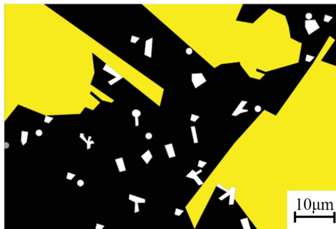
Figure 8. Fugitive state of sulfur in the original slag sample (yellow-matrix phase, black-silicate phase (C3S), white - CaS)
