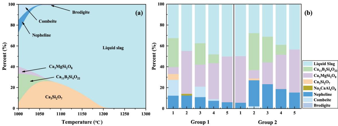
Figure 5. Equilibrium phases of fluorine-free mold fluxes for (a) sample  $\text{MgO}=4$  wt% in Group 1 during cooling process and (b) all samples at 1000 °C
