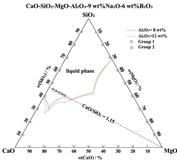
Figure 1. Isothermal section diagram at 1300°C of  $\text{CaO-SiO}_2\text{-MgO-Al}_2\text{O}_3\text{-9 wt\%Na}_2\text{O-6 wt\%B}_2\text{O}_3$  system with various  $\text{Al}_2\text{O}_3$  of 8 wt% or 12 wt%
