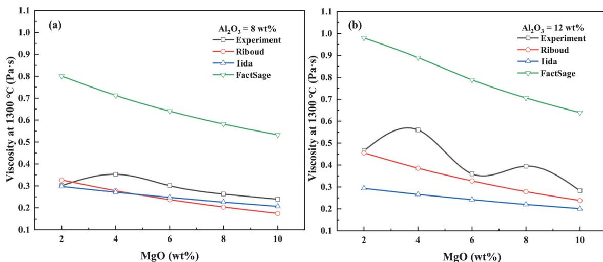
Figure 2. Viscosity at 1300°C of fluorine-free mold fluxes for (a) Group 1 and (b) Group 2
