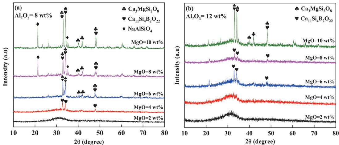
Figure 6. XRD results of fluorine-free mold fluxes for (a) Group 1 and (b) Group 2
