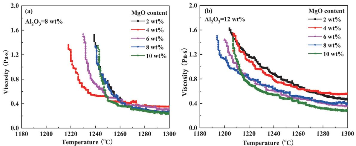
Figure 4. Viscosity-temperature curve of fluorine-free mold fluxes for (a) Group 1 and (b) Group 2
