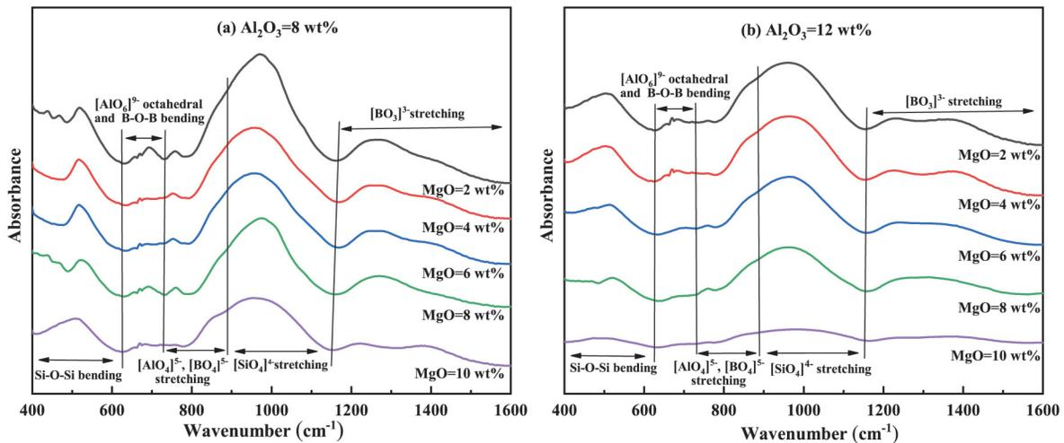
Figure 3. FTIR spectra of fluorine-free mold fluxes for (a) Group 1 and (b) Group 2
