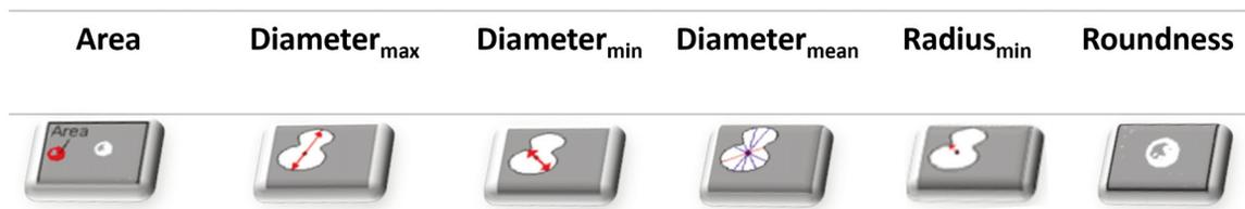
Figure 4. Graphical presentation of selected and monitored parameters
