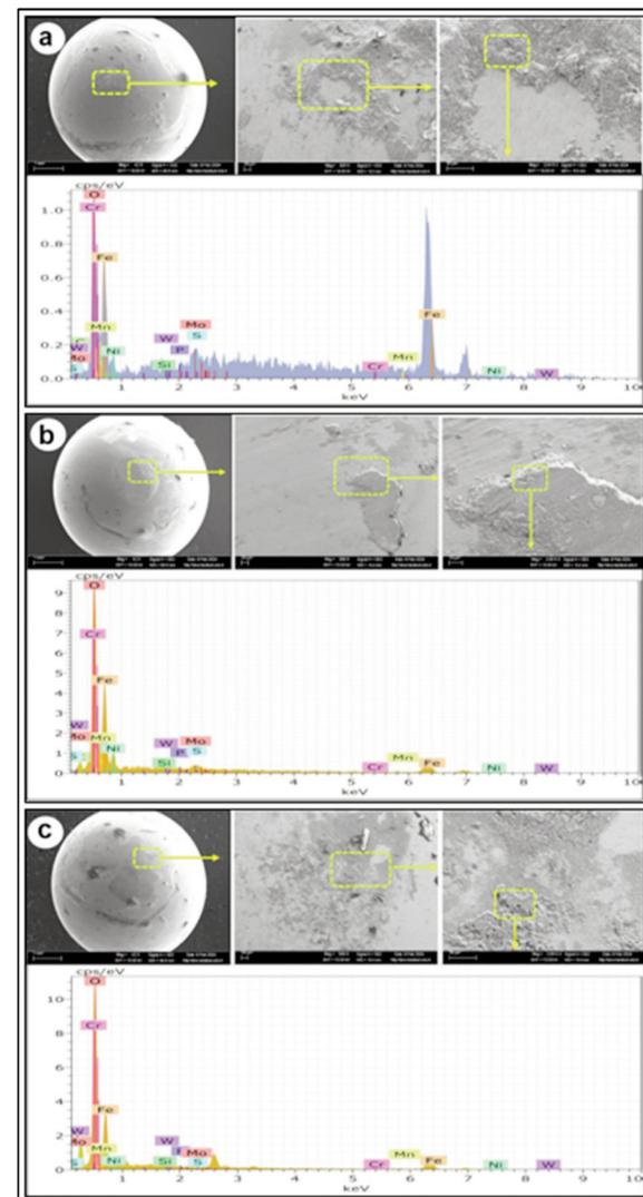
Figure 8. SEM and EDX analysis of abrasive balls of the test carried out at 40N load: a) Undeformed, b) 40% deformed, and c) 80% deformed
