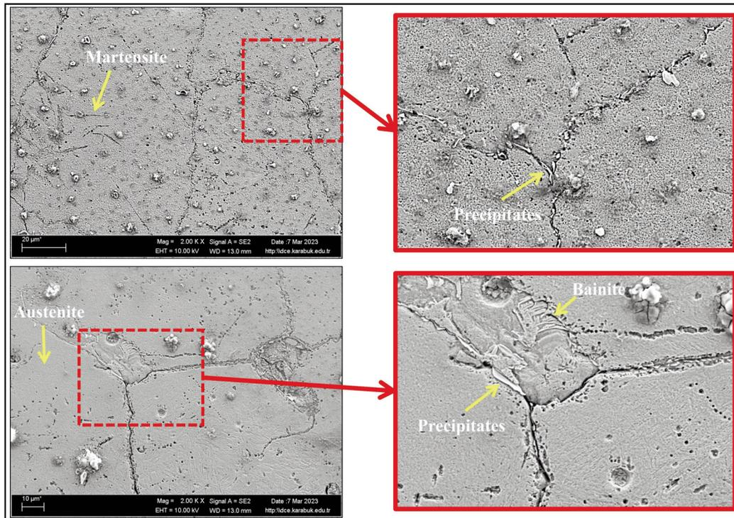
Figure 1. Microstructure details for undeformed sample (2000x-5000x)
