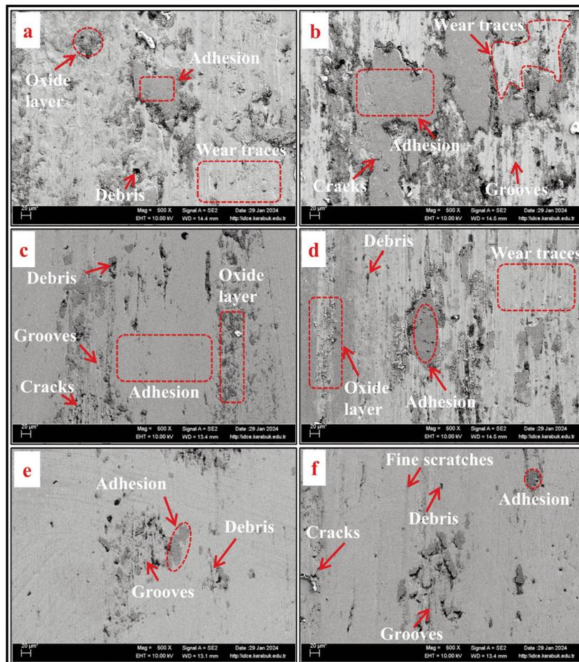
**Figure 6.** Worn surface images of alloys: a) undeformed 20N, b) undeformed 40N, c) 40% Deformed 20N, d) 40% Deformed (40N), e) 80% Deformed (20N), and f) 80% Deformed (40N)
