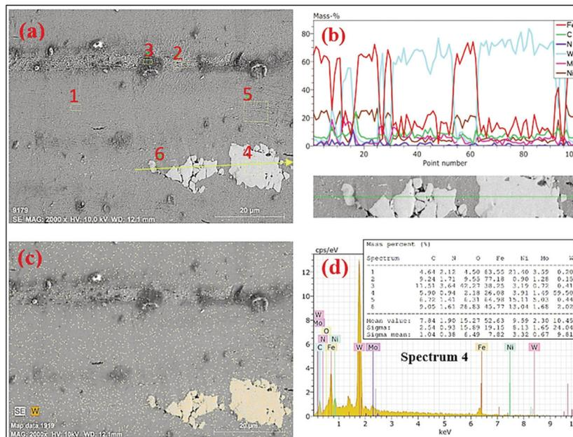
Figure 3. Mo-Ni-W steel 80% Deformed (a, b, and d) SEM point EDS images, and line EDS analysis (2000x), (c) SEM mapping images (2000x)
