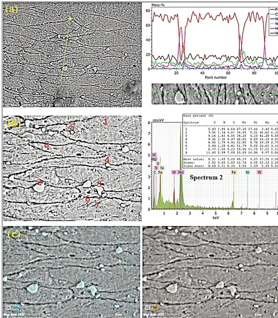
Figure 4. Mo-Ni-W steel 80% Deformed (a) SEM. Line EDS images (10000x), (b) SEM point EDS analysis of precipitates formed in the grain and grain boundaries (20000x), and (c) mapping images of Mo and W
