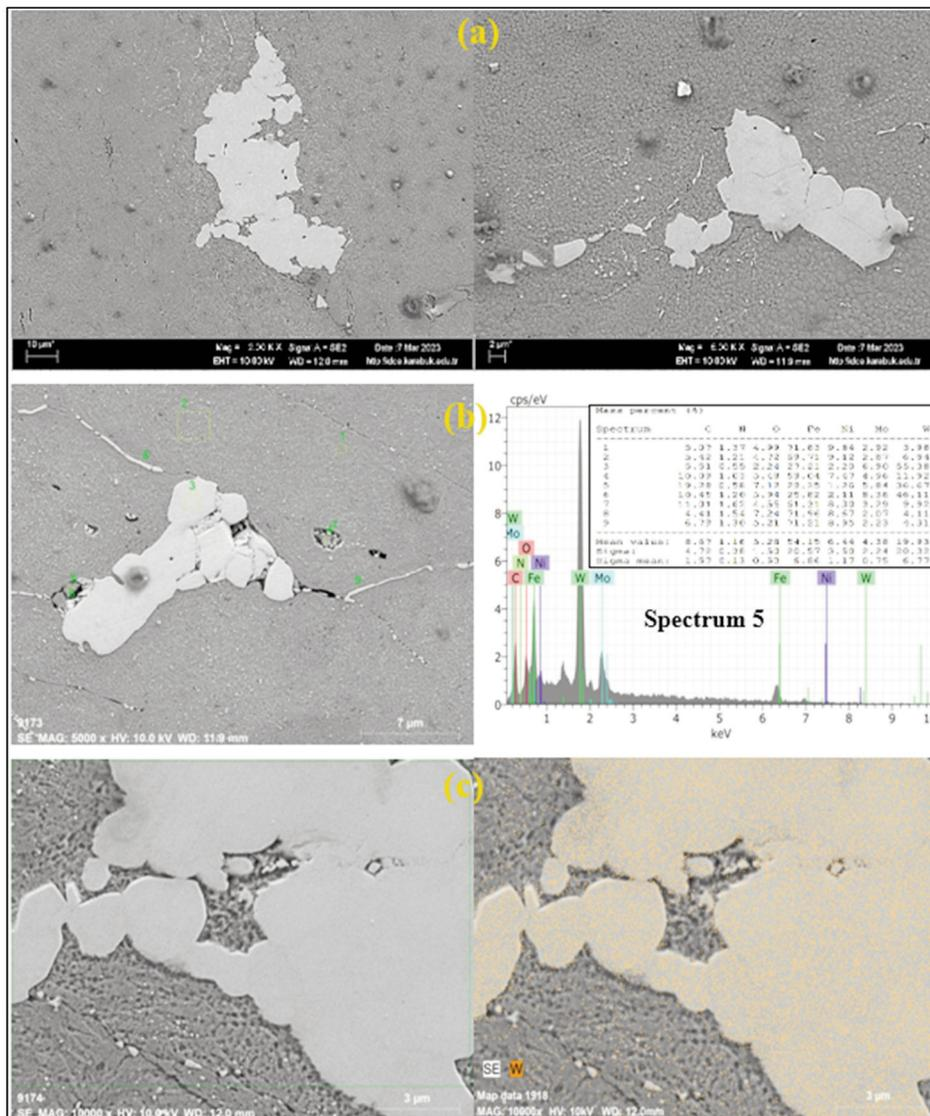
Figure 2. Mo-Ni-W steel 40% Deformed (a) SEM Microstructure images (2000x-5000x), (b) SEM point EDS analysis (5000x), (c) SEM mapping images (10000x)
