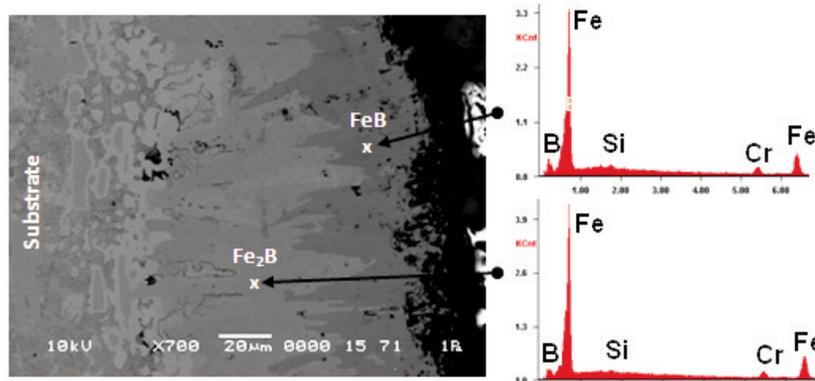
Figure 3. SEM image coupled to the EDS analysis of the cross-section of borided layers formed on the 200CrMoV12 steel at 1000°C for 6 h of treatment.
