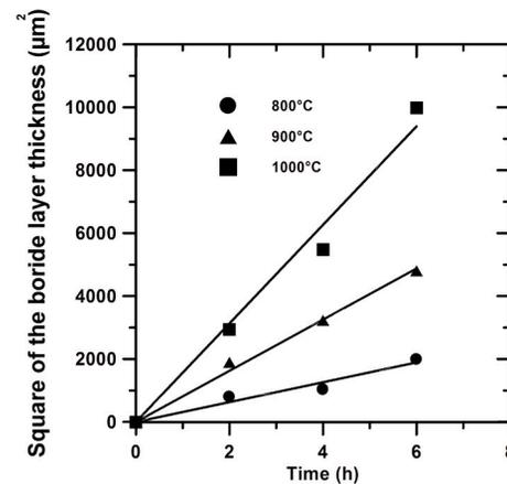
Figure 5. Evolution of the square of boride layer thickness versus time for increasing temperatures.
