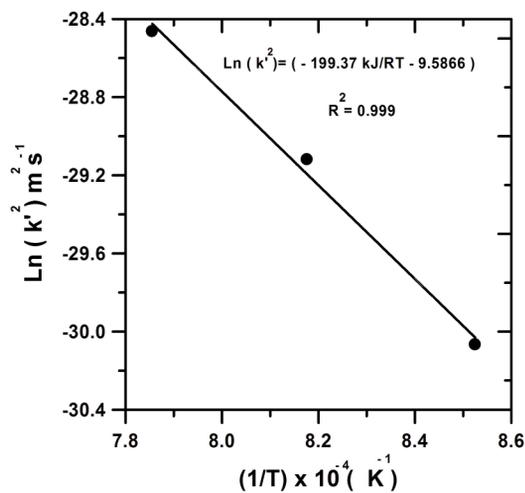
Figure 6. Temperature dependence of the square of parabolic growth constant.
