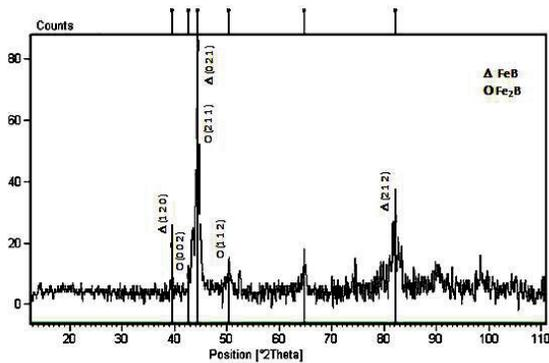
Figure 4. XRD pattern obtained at the surface of borided X200CrMoV12 steel at 1000°C for 6 h of treatment.
