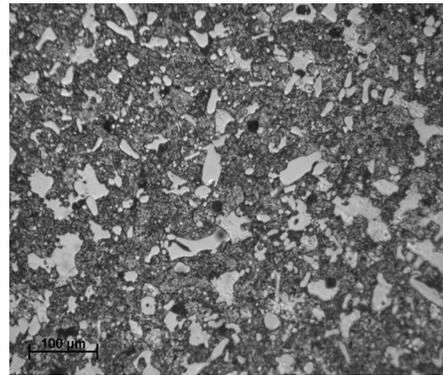
**Figure 1.** Optical image of the initial microstructure of X200CrMoV12 steel after a heat treatment (quenching followed by tempering).
