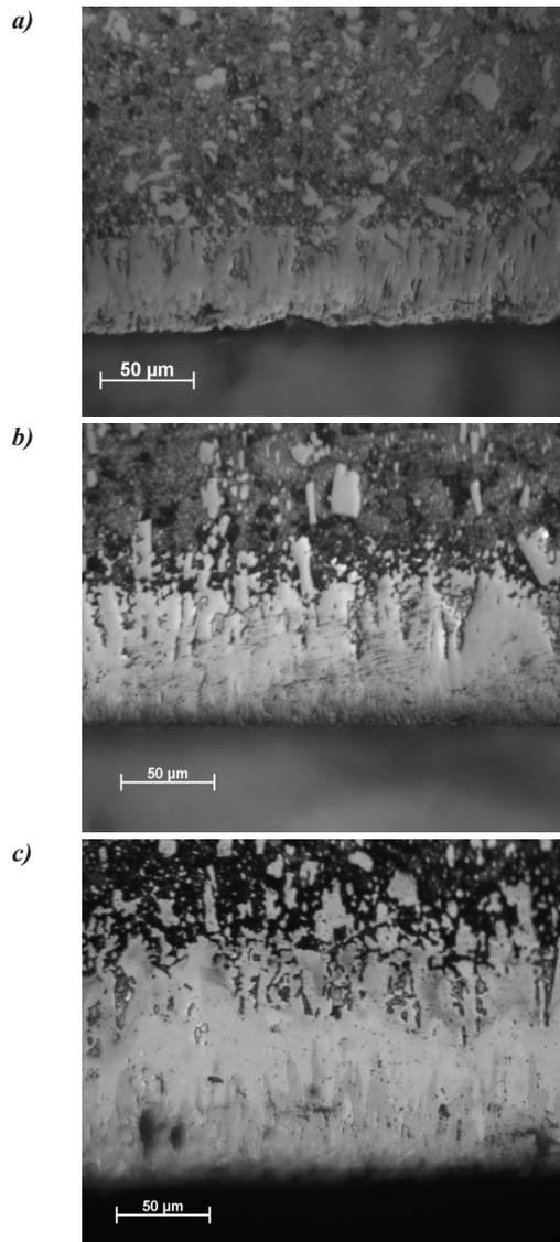
**Figure 2.** Optical micrographs of the cross-sections of the borided layers formed on the 200CrMoV12 steel during 6 h at different temperatures: (a) 900°C, (b) 950°C and (c) 1000°C.
