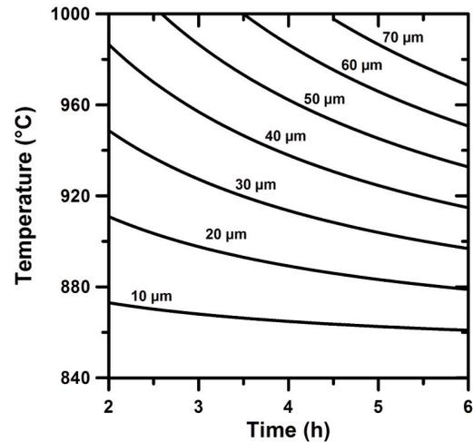
Figure 7. Iso-thickness diagram describing the evolution of the boride layer thickness as a function of the boriding parameters.
