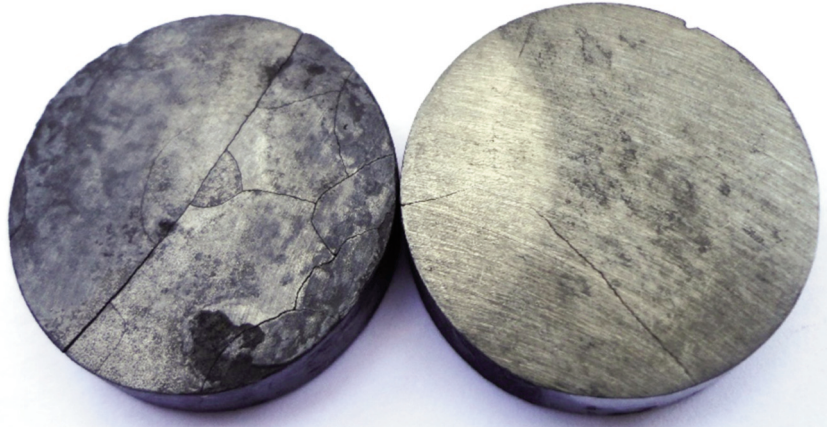
Figure 4. Effect of water quenching after heating AISI T5 to 1200\text{ }^{\circ}\text{C}
