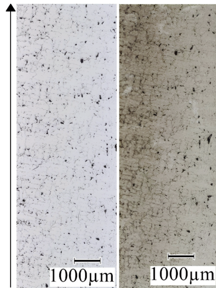
Figure 9. Unidirectional structure, growth velocity v = 5.56 \cdot 10^{-6} m/s; on the right, etched with Nital
