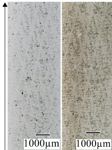
Figure 10. Unidirectional structure, growth velocity a) v = 8.33 \cdot 10^{-6} m/s; on the right, etched with Nital
