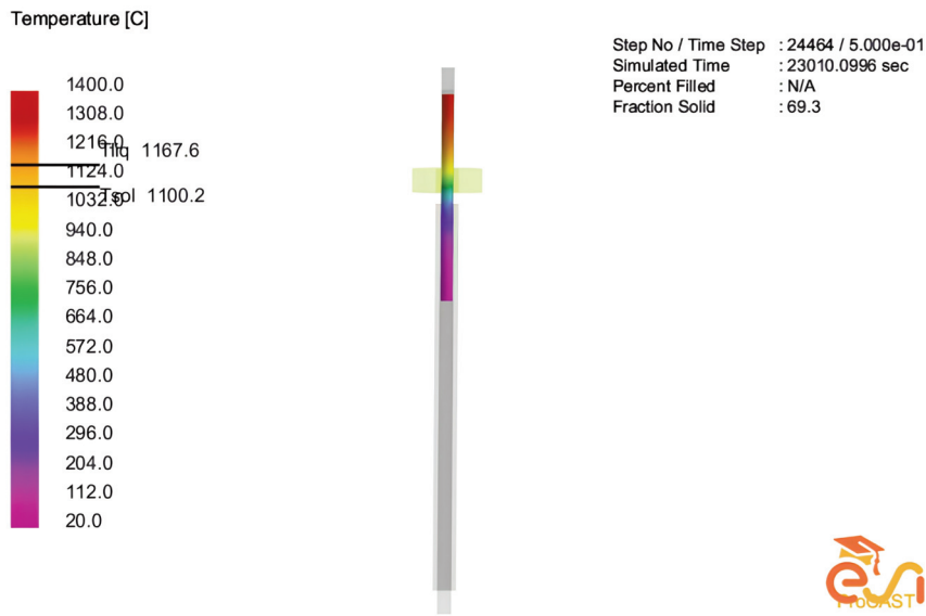
Figure 3. Simulation in ProCAST software - temperature distribution in the sample with the whole system, growth rate v = 2.5 \cdot 10^{-6} m/s (liquidus temperature 1167.6 °C, solidus temperature 1100.2 °C)
