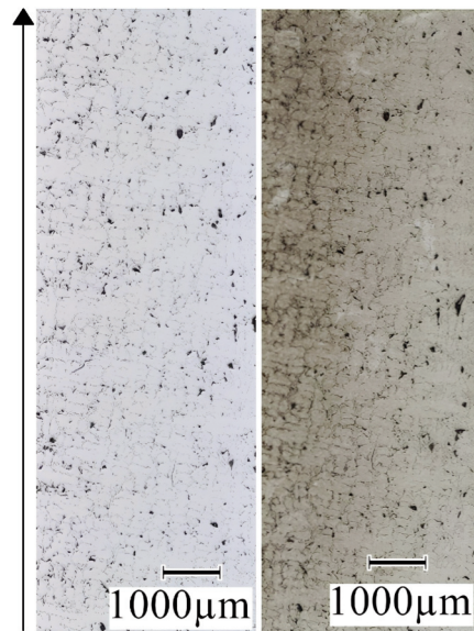
Figure 11. Unidirectional structure, growth velocity a) v = 1.11 \cdot 10^{-5} m/s; on the right, etched with Nital
