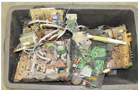
**Figure 1.** Input material for mechanical pretreatment experiments
